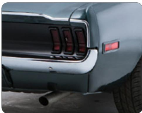
The exhaust system is up to you. Different brands have different sounds, but a totally straight-through system is likely to be uncomfortably noisy. The important visual element, though, is to make sure that the pipe is cut straight where it exits beneath the rear bumper. Certainly, any fancy tips should be removed.
