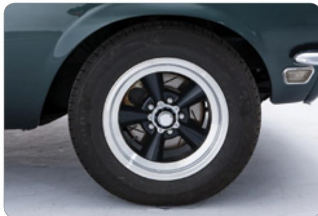
Off the production line, a '68 Mustang would have worn 14" x 5" wheels, although Shelby cars wore 15" wheels.
